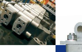
ABCO Subsea patented the first Multi-Input Shuttle Valves for the offshore industry more than 30 years ago. The valves are manufactured with two to seven input ports.
