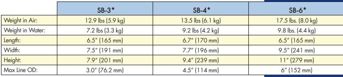
\*Measurements include Clamp assembled with an adapter bracket.
