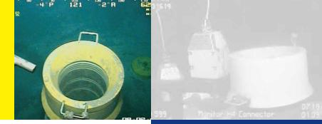
ABCO Subsea is bringing to market a Subsea Wellhead Guide Funnel. The Funnel protects the ring gasket sealing surface on high pressure subsea wellheads, BOP stacks and horizontal subsea trees during open-water work. The Funnel facilitates wellhead tools entering the wellhead.
