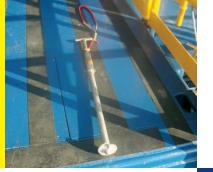
ABCO Subsea is bringing to market an ROV-operated Valve Cleanout Tool. Subsea wellhead Valves often become plugged with gumbo while the conductor hole section is being drilled before the riser is in place. The ROV-operated Valve Cleanout Tool fixes this problem.
