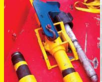
ABCO Subsea is bringing to market a Ball Valve Handling Tool to help eliminate manual handling of heavy loads in the moon pool. This tool can be mobilized by a single deckhand and is load tested per the operator's lifting policy.
